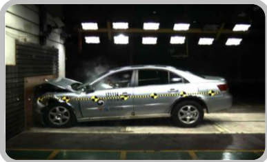
Frontal-impact test striking a wall head on
