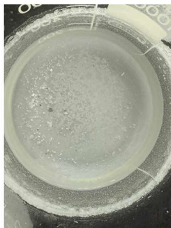
< Chemical precipitation of \text{Li}_2\text{CO}_3 after 1 h at 0.5 M \text{LiCl} with 0.3 M \text{Na}_2\text{CO}_3 >
