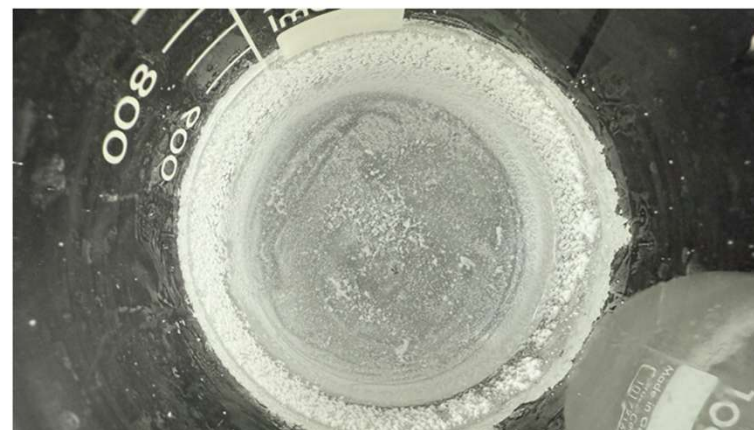
< At 2V, Denser \text{Li}_2\text{CO}_3 precipitation layer forming along the beaker bottom and wall after 1 h at 0.5 M \text{LiCl} with 0.3 M \text{Na}_2\text{CO}_3 >
