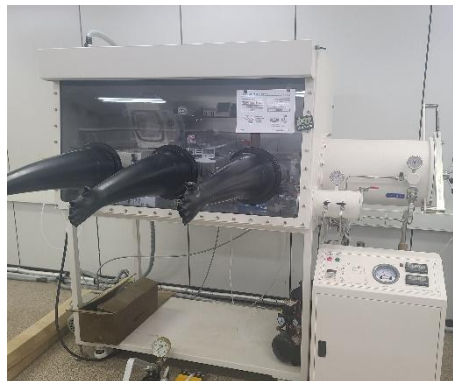
Glove box for electrolyte synthesis
