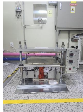
Hot Press for bipolar plate
