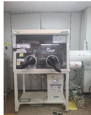
Glove box for cell fabrication
