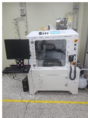
Ultrasonic spray coater
