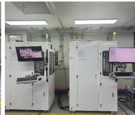
PEMFCs single cell test systems
